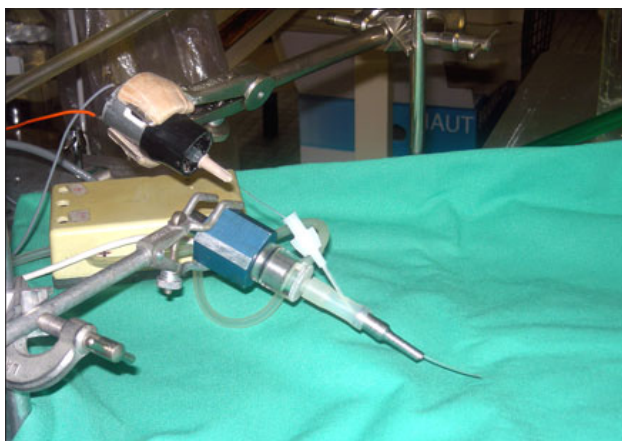
Fig. 1. The system developed for mechanical stimulation of trachea. The rotating probe consisted of the silastic semi-rigid catheter (1) with proximal end connected to a small electrical motor (2) and the distal end placed into the rabbit trachea through the tracheal cannula (3). Fleisch pneumotachograph (4).
